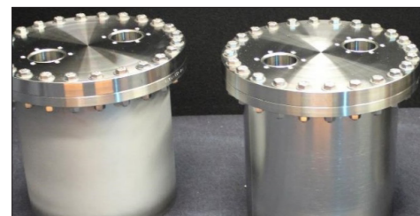
Size matters: using vacuum chambers with the same geometry enables a better comparison of outgassing rates (Courtesy: Anderson Dahlen).
