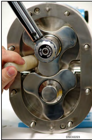
Figure 69 - Tighten rotor nuts
