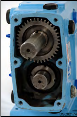
Figure 60 - Install timing gear on drive shaft
