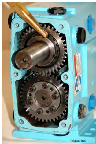
Figure 71 - Bend tab into locknut slot
