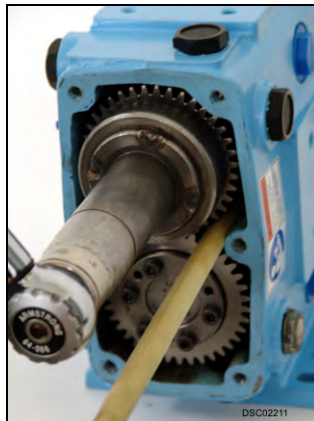
Figure 70 - Tighten and torque drive shaft
