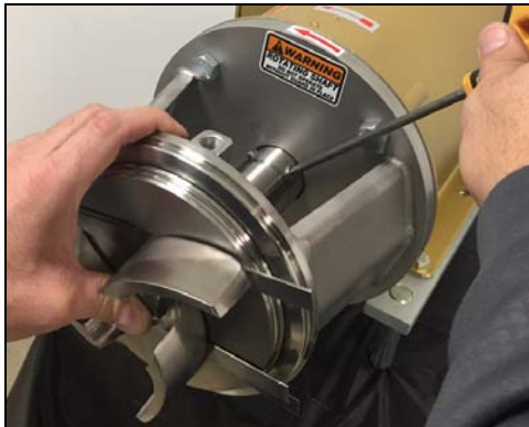
Figure 37 - Place feeler gauge, tighten setscrews
