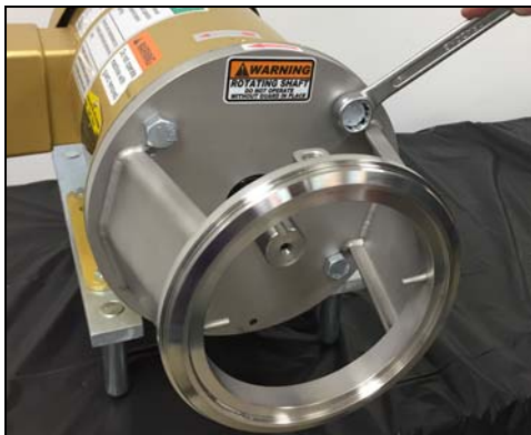
Figure 78 - Install motor adapter bolts
