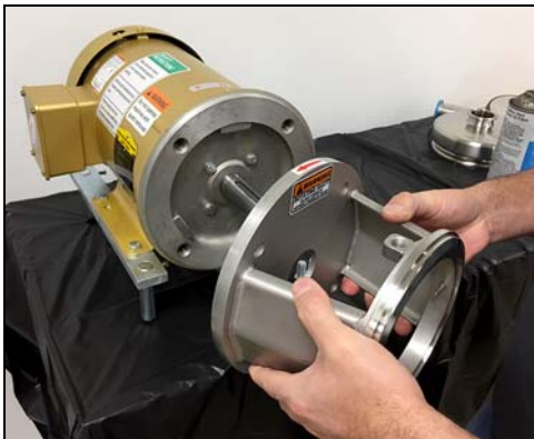
Figure 26 - Remove motor adapter
