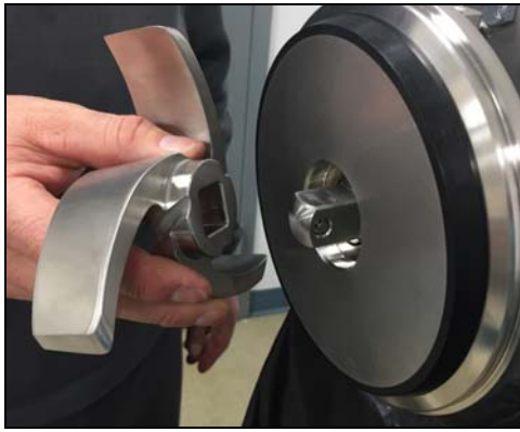
Figure 35 - Slide impeller on shaft
