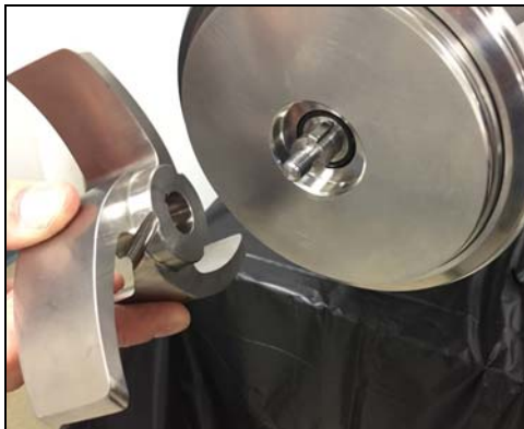
Figure 107 - Install impeller on stub shaft
