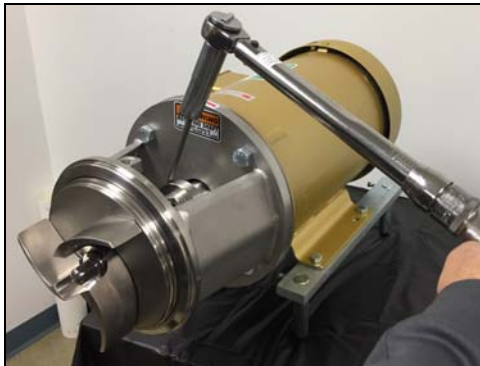
Figure 92 - Torque drive collar screws
