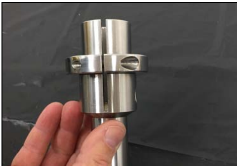
Figure 81 - Slide drive collar on stub shaft
