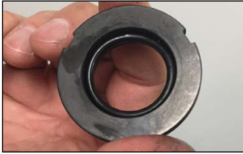
Figure 43 - Seal O-ring installed
