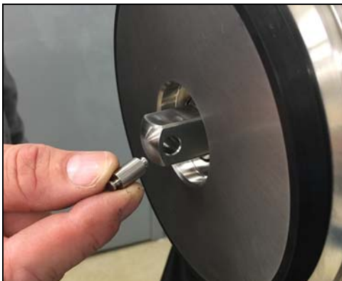
Figure 33 - Insert impeller retainer pin
