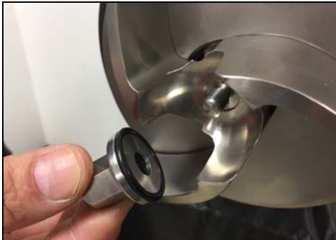
Figure 109 - Install impeller nut
