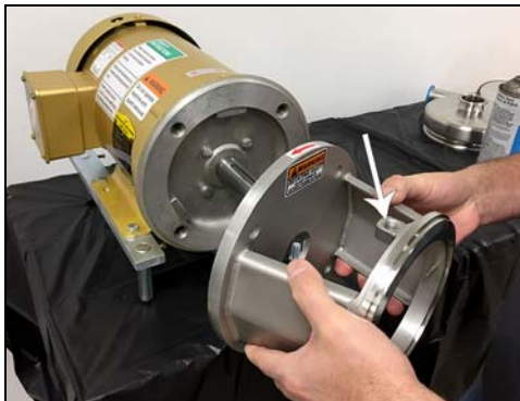
Figure 77 - Install motor adapter
