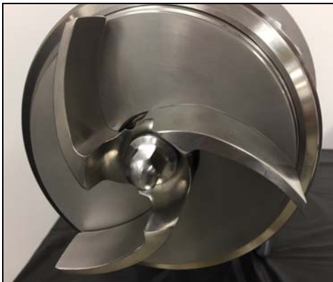
Figure 110 - Hand-tighten impeller nut
