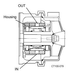
Figure 19 - Type 4 Liquid Flush
