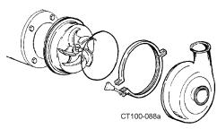
Figure 35 - Install Casing
