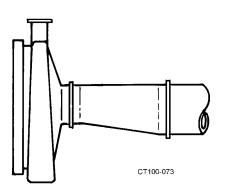
Figure 15 - Correct Eccentric Installation
