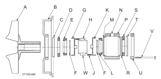
Figure 38 - Type 4 Seal Components
