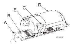
Figure 58 - Typical Cartridge Seal
