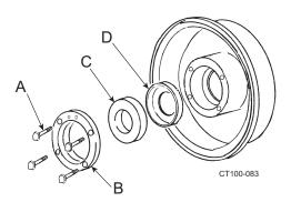
Figure 27 - Removing Stationary Seal
