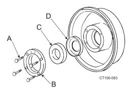
Figure 29 - Stationary Seal Assembly
