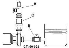
Figure 21 - Pump Below Supply (Feed Source Above Pump Level)
