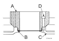
Figure 54 - Insert L-gasket, Fasten Adapter in Place
