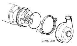
Figure 43 - Install Casing
