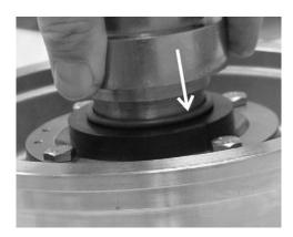
Figure 40 - Installing O-ring Using Spring Retainer
