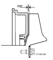
Figure 33 - Clearance Between Impeller and Backplate
