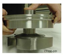
Figure 37 - Move Rotary Seal Up Shaft
