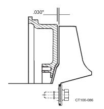
Figure 41 - Clearance Between Impeller and Backplate
