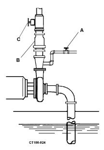
Figure 22 - Pump Above Supply (Feed Source Below Pump Level)
