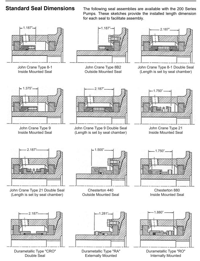
Figure 64 - Installed Standard Seals (length provided for aid of assembly)
