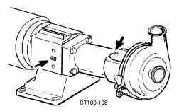
Figure 60 - Grease Fittings on the Pedestal Pump
