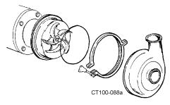
Figure 59 - Install O-ring, Casing, Clamp
