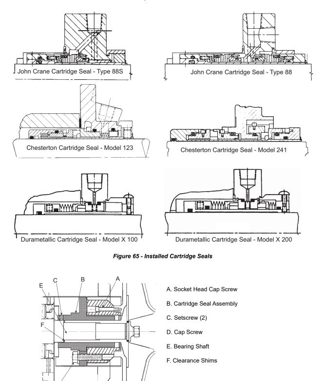
Figure 66 - Typical Cartridge Seal Installation
