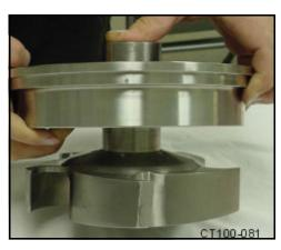
Figure 25 - Moving Rotary Seal Up the Shaft
