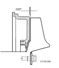
Figure 53 - Clearance Between Impeller and Backplate
