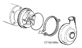
Figure 50 - Remove Casing Clamp, Casing and O-ring
