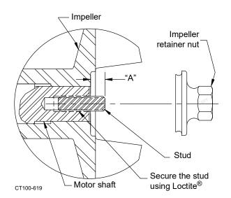
Figure 63 - Replacing the Impeller stud and nut
