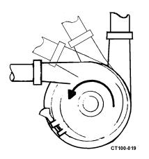
Figure 13 - Recommended Discharge Positions
