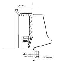
Figure 39 - Shim Placement
