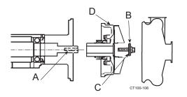
Figure 57 - Installing Impeller Assembly
