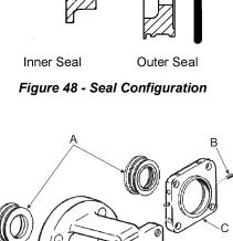
**NOTE:** Replace all rubber parts whenever a unit is dismantled for inspection or repair. Lubricate the rubber parts with an approved/ sanitary lubricant prior to assembly.
