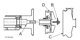
Figure 44 - Removing the Impeller Assembly
