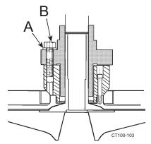
Figure 55 - Fastening Seal Unit in Place
