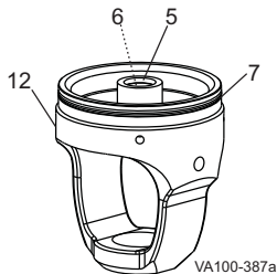
Figure 33: Remove Yoke O-ring and Guide Bearing
